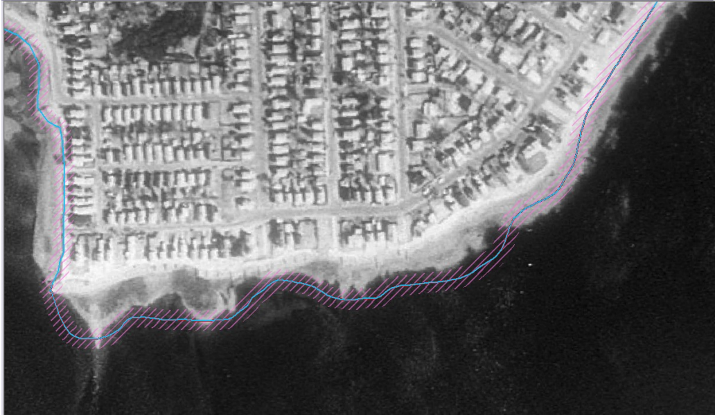
Figure 3: Examples of suitable (top) and unsuitable (bottom) shoreline vectors.
